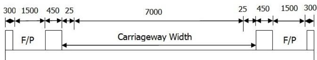
Bridge Cross Section with Footpath
